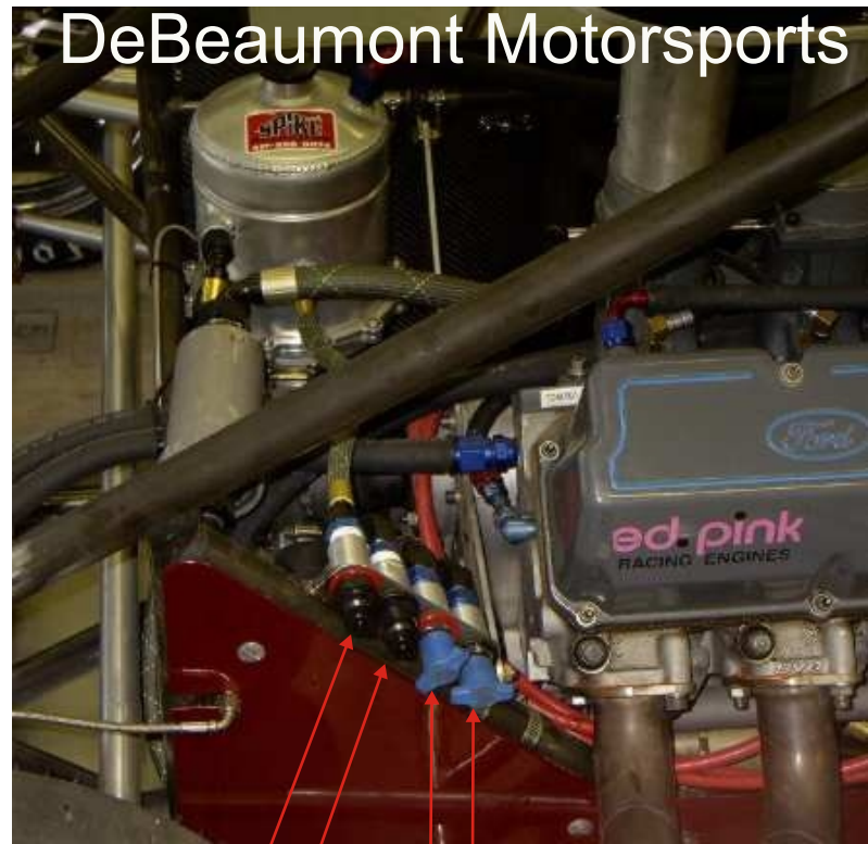
Oil Heater Connections Hot Oil To Oil Tank Cold Oil From Oil Tank Engine Coolant Heater Connections Hot Water Out Hot Water In
